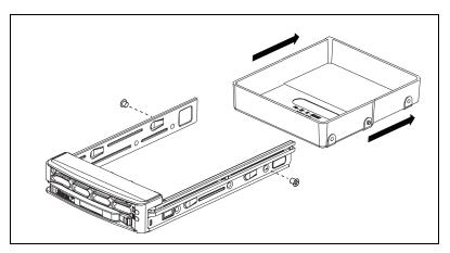
Figure B-26. Removing Dummy Tray
